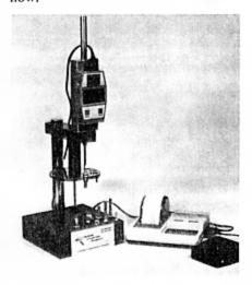
All military fastener flat heads are measured in cylindrical gage diameters. One minor difference is that the indicator foot (stylus) is to be of a forked design so that the foot will straddle the recess unlike the commercial approach with a flat foot that rests across the entire screw head. The military specifications sometimes refer to this head feature as "flushness" instead of "protrusion".
