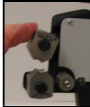
5. Insert the GO plug between the segments and rotate the set plug clockwise slightly to assure the plug is completely seated in the segments.
