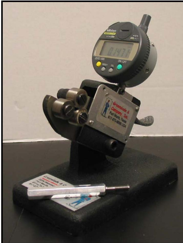
3. Without doing anything else to the gage, change the pre-set value to the value displayed while the gage arm is at rest without the setting plug in the gage.
