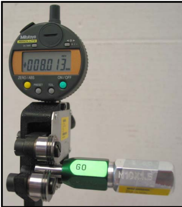
Setting indicator for inspecting The thread minor diameter
