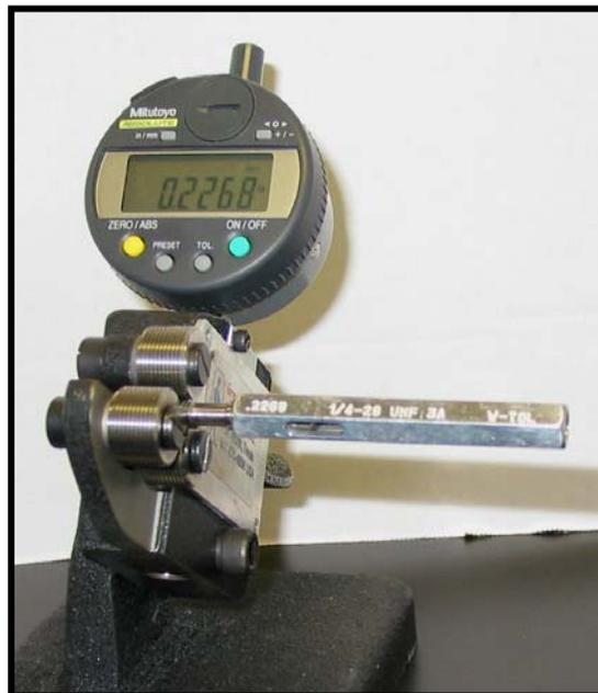
5. Remove the setting plug and the retaining screws on the bottom two roll axis pins.
