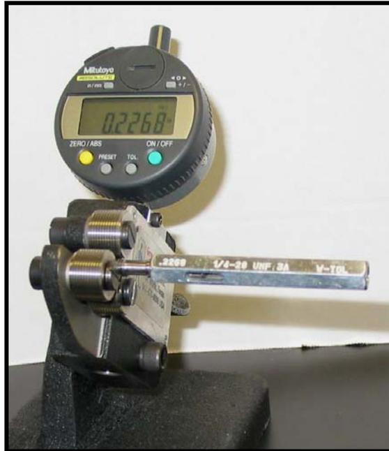
2. Remove the setting plug and record the indicator value displayed on the indicator when the arm is in its resting position.
