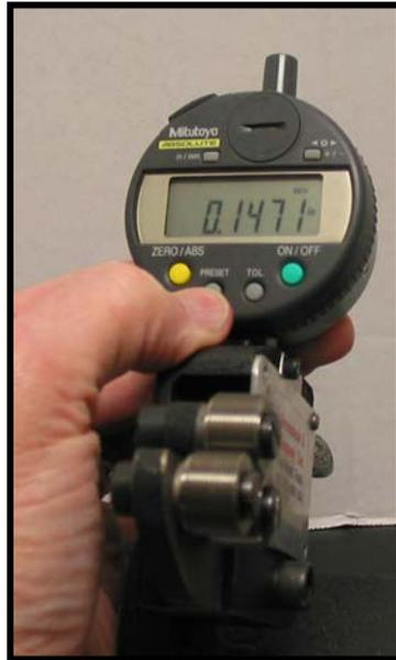
4. Open the gage and place the setting plug between the rolls and slightly rotate the plug to assure its full seating between the rolls. The reading displayed on the indicator should be that of the setting plug size.
