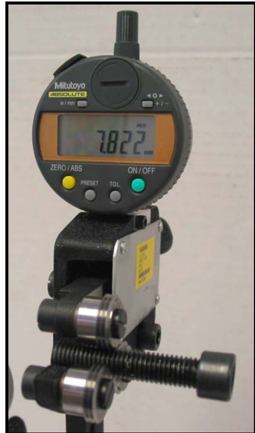
Inspecting the thread's minor diameter
