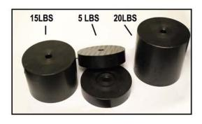
1. Select the correct weight for the test to be conducted and place it on the vertical weight holding post on the left end of the lower arm of the test fixture.
