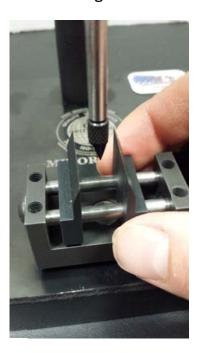
2. Lift the upper knife edge probe out of the way, and place the fastener onto the lower knife edge anvils. Make sure to settle the anvils into the thread grooves, and drop the upper knife edge probe into the groove on the top side of the fastener.
