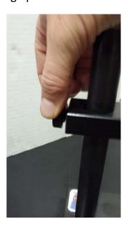
2. Move the lower knife edge anvils apart as far as they will go and place the .200" diameter setting pin across them approximately in the middle. Drop the upper knife edge probe onto the top side of the master setting pin.
