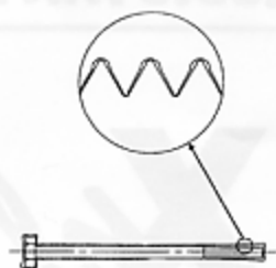
Figure 1. The uneven build-up of electroplated finishes on fasteners.
