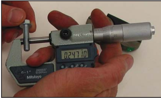
Inspecting bolt's major diameter.
