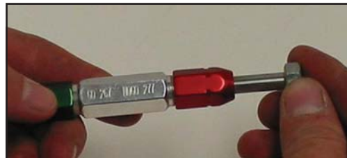
GO cylindrical plug gage enters nut minor diameter.
