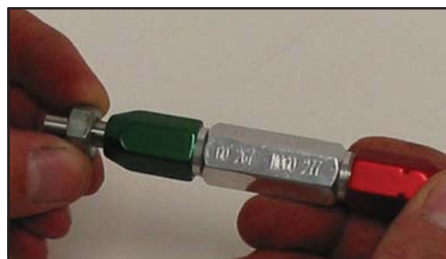
NOGO cylindrical plug gages does not enter nut minor diameter.
