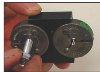
Bolt not entering GO ring gage.
