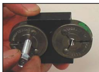
Bolt not entering GO ring gage.
