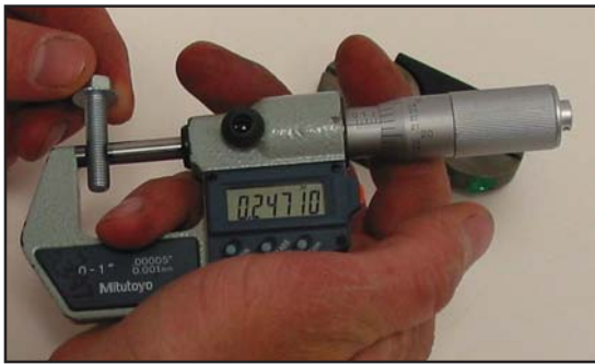
Inspecting bolt's major diameter.
