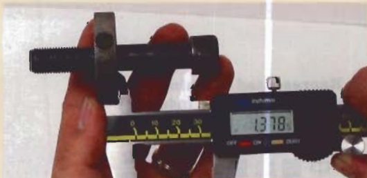
Lg measurement using standard GO ring gage
