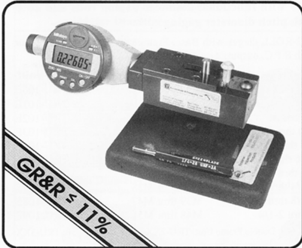
Segment External Thread Gage (ANSI/ASME Gage #4.1)
