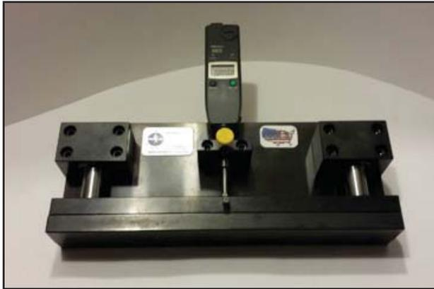
The part is then rotated until the maximum indicator reading is achieved. The reading on the indicator is the exact amount of camber or bow in the measured part. Unlike the fixed jaw style of gage, you do not add the screw diameter to the allowable bow. Using this style of
