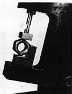
Measuring nut across corners (AC).
