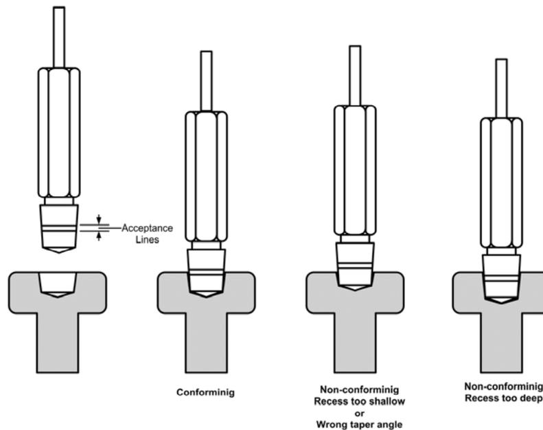
A good square socket recess will cling to the fit gage. To inspect for “cling”, press the screw on to the gage point while holding both horizontally and without holding the screw on to the gage, turn the gage horizontally with the point of the gage pointing downward. The fit is acceptable if the screw clings or sticks on the gaging point.
