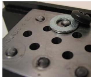
5. Calculate the hydrogen embrittlement test torque for the particular tapping screw lot being evaluated by first determining the average of the five failure values and then by multiplying that average by 80%. As the example in the photographs shows, the average failure value was 200 inch pounds. The test torque is then 160 inch pounds (200 X .8).
