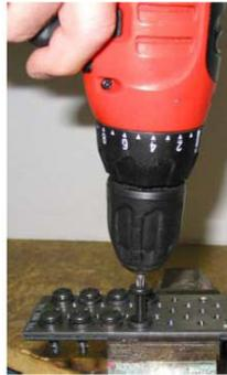
4. Place the test plate in a test fixture and tighten five of the test screws using a calibrated torque wrench until the screws twist into two pieces or until the screws strip out of the test plate. Record the torque value at which each of the five screws failed.
