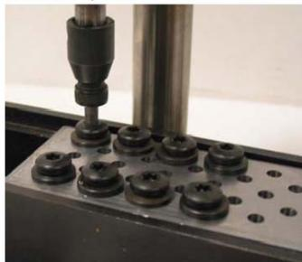
7. Let the samples sit for 24 hours and then re-apply the same torque value as was originally applied 24 hours earlier in the same clockwise (tightening) direction. If no screws break either before the torque is re-applied or while it is being re-applied the tested lot has a very high probability of not having hydrogen embrittlement.
