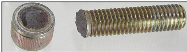
1. The failure must be a DELAYED failure. The delay is generally from one to 24 hours after installation. If the failure occurs during installation, it is definitely NOT caused by hydrogen embrittlement.
